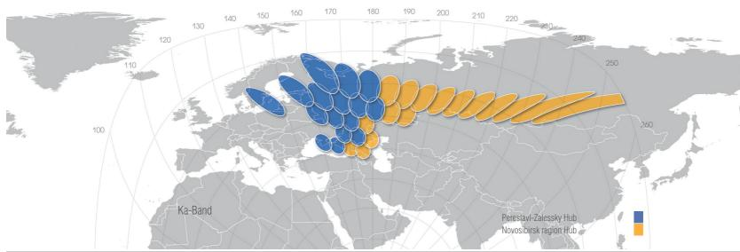
The multi-beam service zone in Ka-band will cover the most populated part of the territory of Russia, reached from 49° E position (European part of Russia, including Kaliningrad region, the Urals, Western Siberia). The system in Ka-band allows to provide economical high-speed broadband services to corporate sector, regional administrations, small businesses and individuals.
